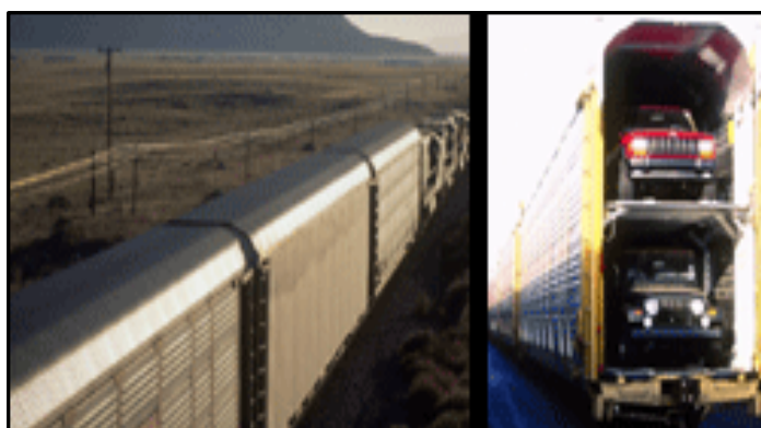
Bi-Level Auto Rack - 94 feet and 10 medium size automobiles
