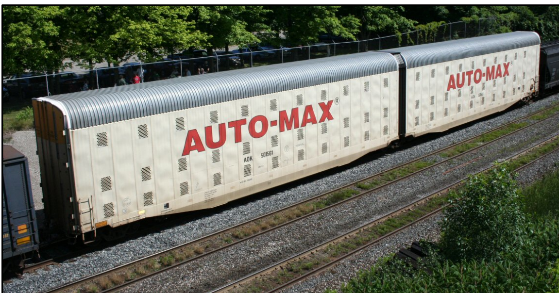
Auto Max Auto Rack - 141 feet and 24 vehicle capacity
