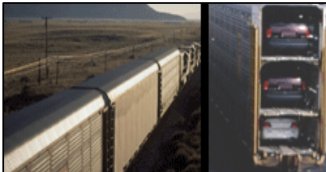
Tri-Level Auto Rack – 94 feet and 15 medium size automobiles
