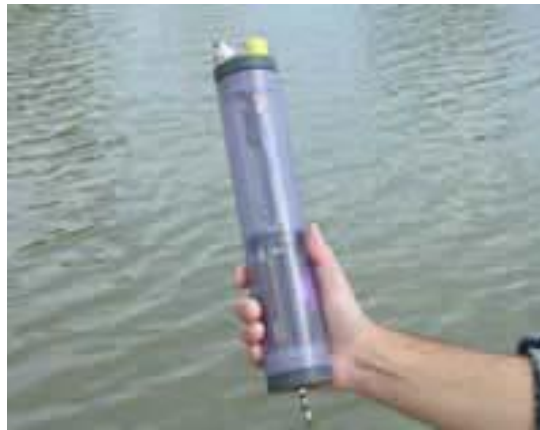
Figure 1. Submersible ultrasonic receiver (SUR; Sonotronics, Tucson, AZ).
