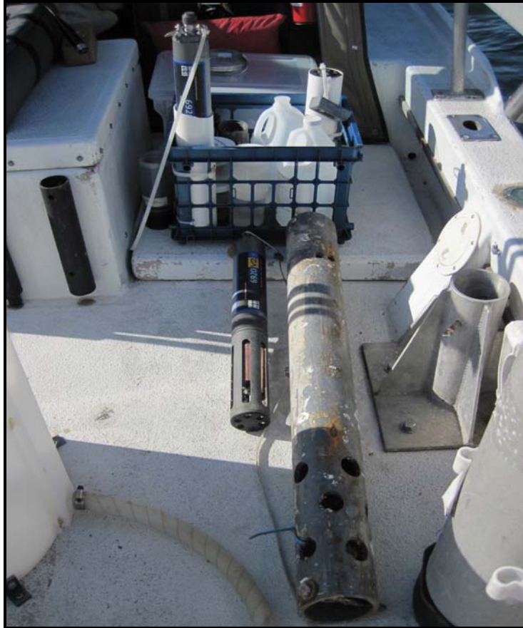
Photo 2. YSI 6920 V2 Sonde and PVC housing used to reduce fouling, prior to installation on buoy mooring chains.
