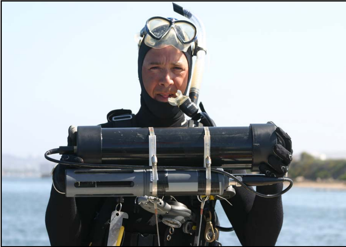
Photo 2. Diver prepares to install YSI sonde at Station A.
