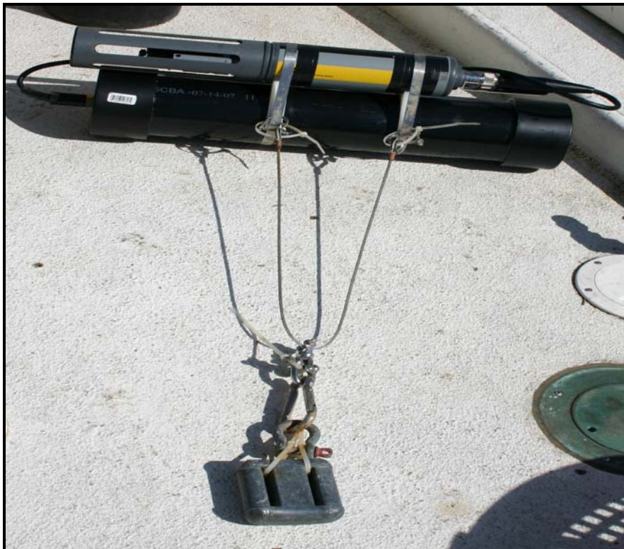
Photo 2. YSI sonde with stainless rigging (weight is removed once the unit is affixed to the bottom).
