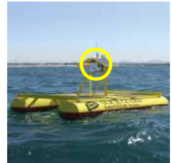
Figure 5C. Slick Guard Environmental Platform w/ Slick Sleuth Sensor, Wireless Radio (900 MHz) and Solar Power.
