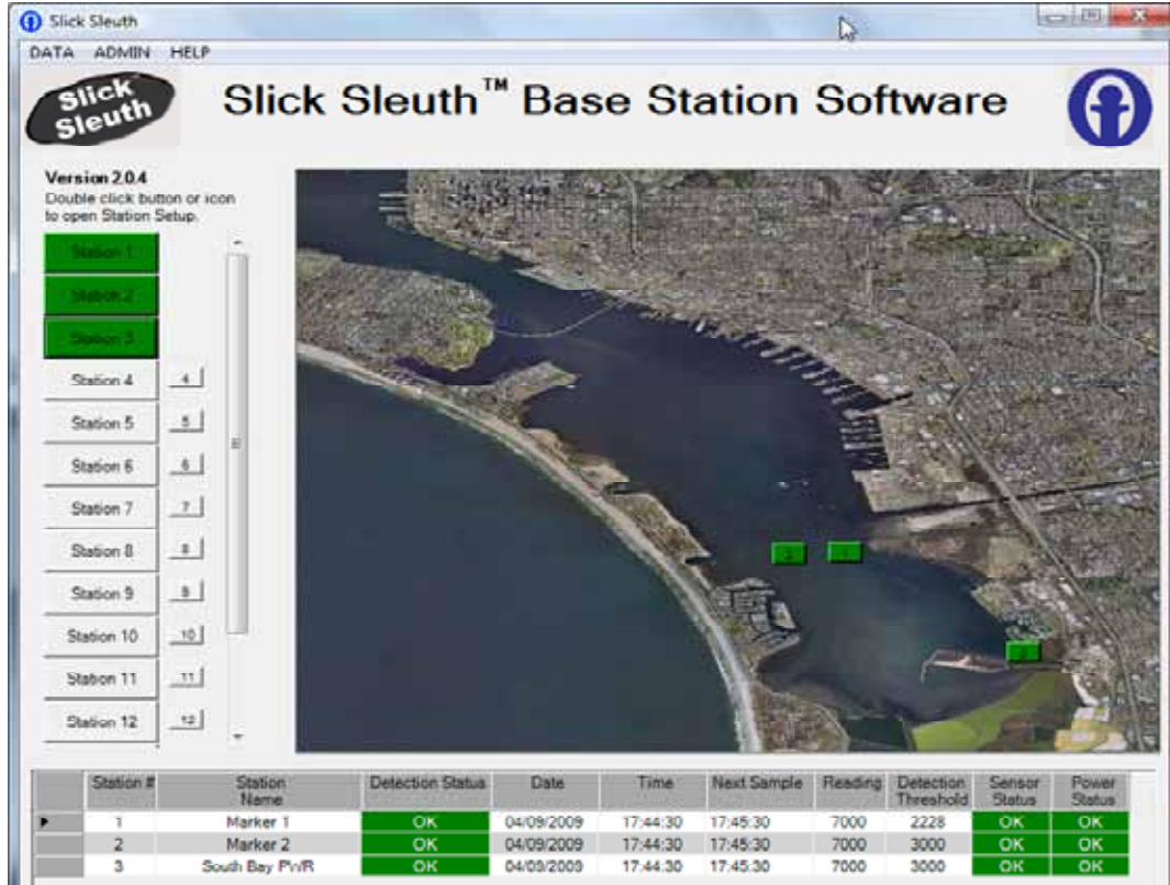
Figure 4. Sample Screen Capture of Slick Sleuth Base Station. In addition to Real Time Data and Alarm, Every Sampling the System Reports & Archives: Station Name, Oil Detect/No-Detect, Date & Time Stamp, Actual Measurement, Sensitivity Setting, and System Diagnostic Health.
