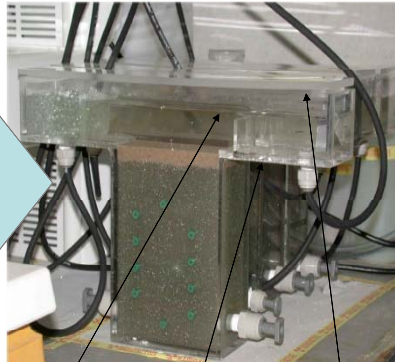
Photograph of Reactive Cap Barrier over Sediments Test Apparatus
