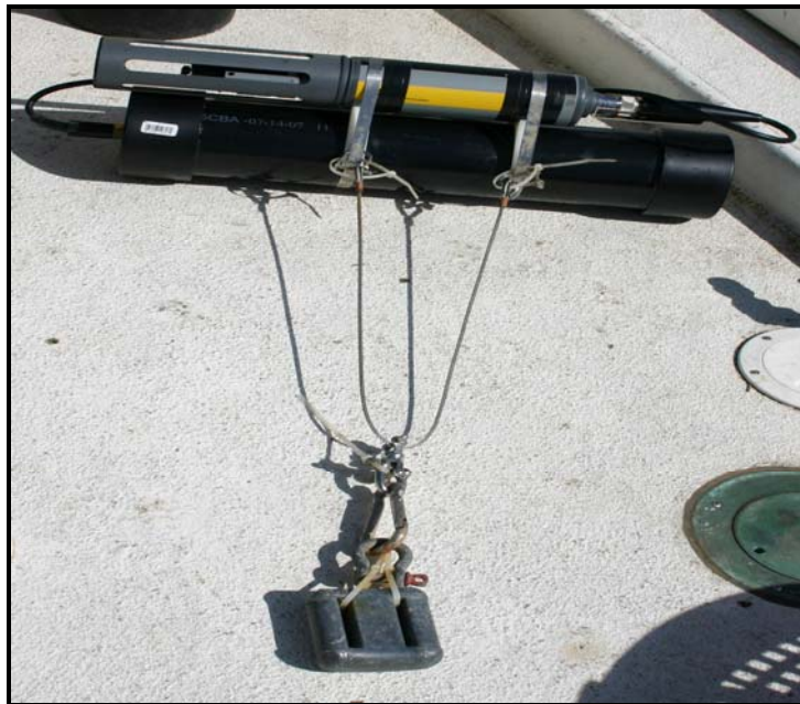
Photo 1. YSI sonde with stainless rigging (weight is removed once the unit is affixed to the bottom).
