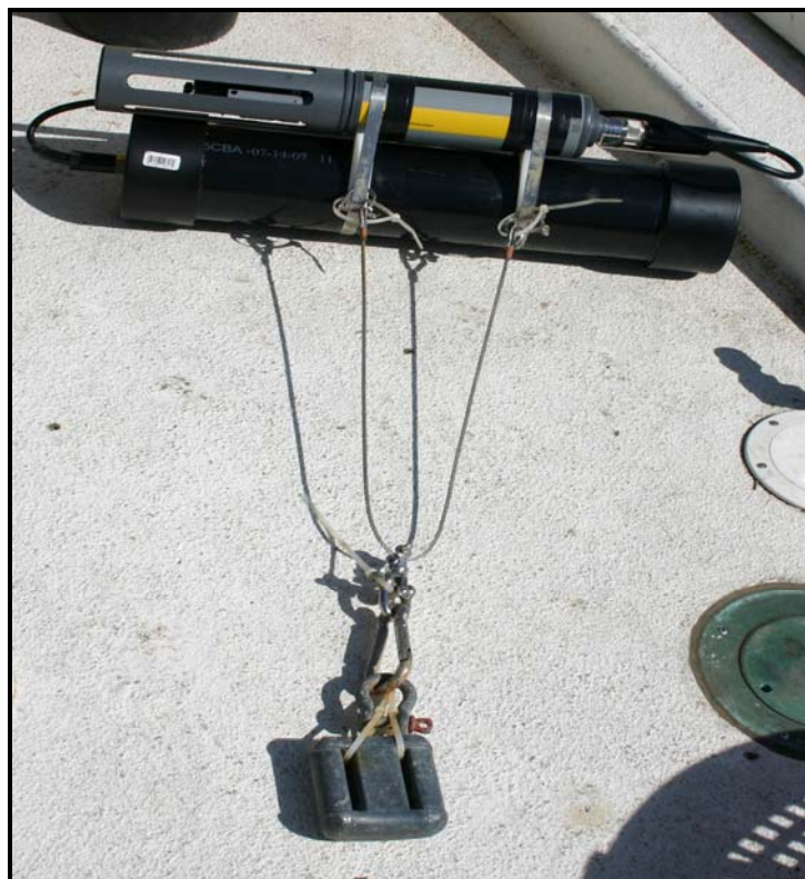
Photo 1. YSI sonde with stainless rigging (weight is removed once the unit is affixed to the bottom).
