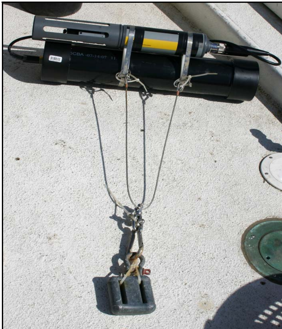
Photo 1. YSI sonde with stainless rigging (weight is removed once the unit is affixed to the bottom).
